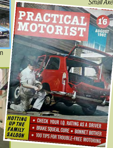
Steve Stone spotted this front cover from 1962. Worryingly, the mechanic is relying on the A40's standard jack to support it. Older members will no doubt recall that the door cannot be closed while the jack's in use, and there are probably some unfortunates whose sills were rusty enough to bend upwards under the weight of the car, meaning a whole new world of pain 'cos even if the jammed jack could be removed, the door wouldn't close!
