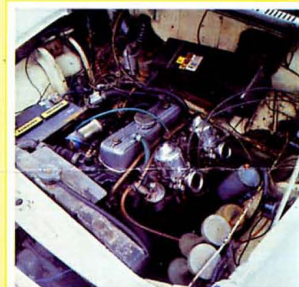
Aluminium rocker-cover and twin carbs are non-standard on this Speedwell-modified 948cc Mk I, as are the twin horns. In September 1962 this engine was replaced by the 1098cc unit.
