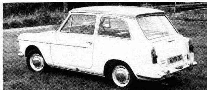
Rear aspect of Mk 2 A40 saloon shows its push-button bootlid handle and the new no. plate light (also seen on late Mk 1s) which replaced the 'button' (Mini-type) used earlier.
