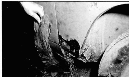
Rotten lower wing hides rusted-out sill, but can be repaired
