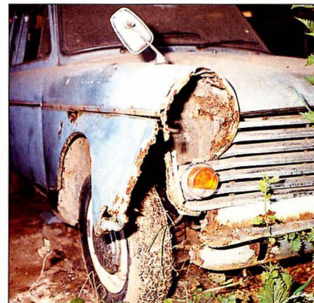
Front wings are particularly prone to rot on all models
